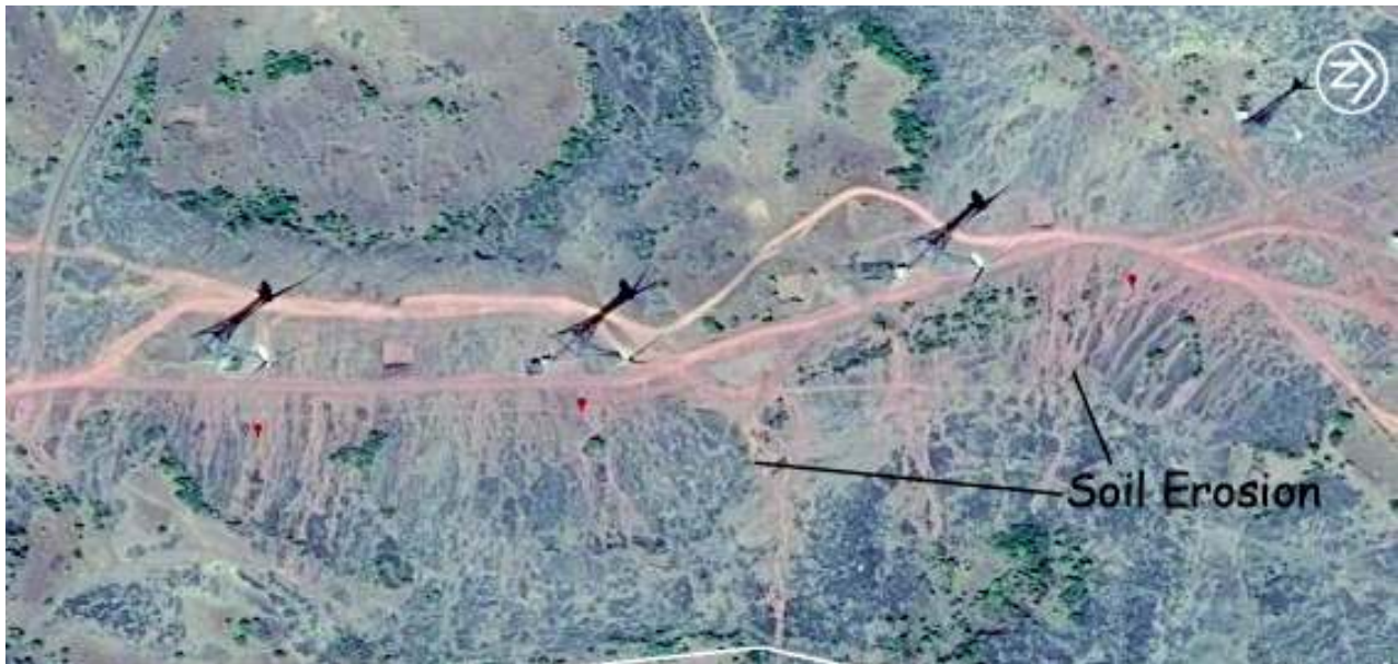
Image 21 : Soil erosion initiated due to road work
